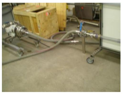
Testing Rig for observing hold up of Sight Glasses
